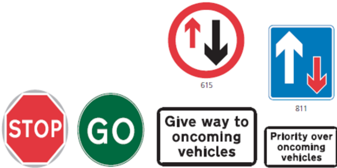
Figure 1.5: Manually operated stop/go signs and priority signs
